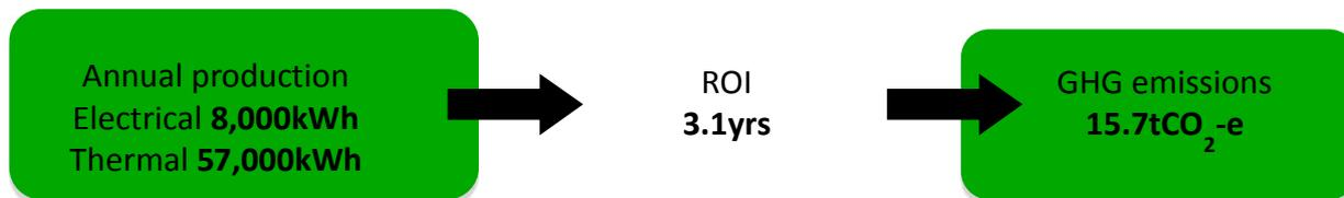
In application for Shaw+Smith this would allow for a reduction in electrical and LPG consumption of 3% and 42% respectively. Additionally this system will reduce the load on the transformer allowing for the projected future growth of the winery and provides a point of difference for marketing.
