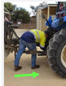
To attach the PTO shaft, step one leg over the lifting arm; adopt a **forward lunge** posture.
