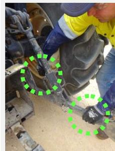
To attach the 3 point linkage, remove pins on the lifting arm stabilisers to align with the implement's linkage points.
