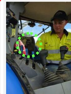
When connecting / disconnecting hydraulic lines ensure you have released the oil first.
